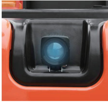
Equipped with LED blue safety light for pedestrian protection.
