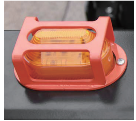
Flashing LED beacon alerts pedestrians during operation.
