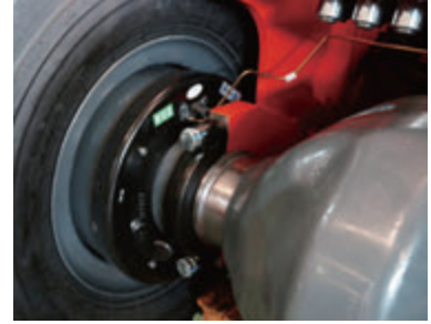
Upgraded drum brakes for improved safety and comfort.
