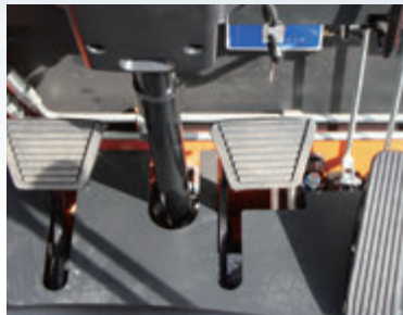
Refined pedal layout for improved comfort (Hydraulic Model).
