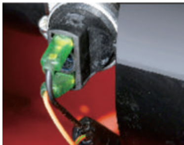
Air filter alarm for timely maintenance and engine protection.
