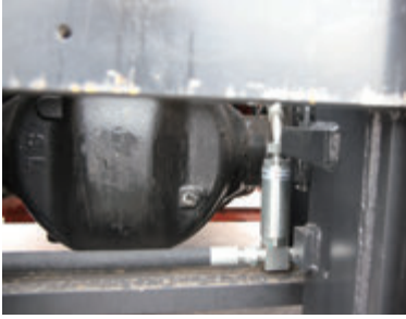
Lift cylinder cushioning for smooth handling.
