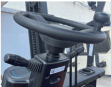
Electro-hydraulic directional switch & multifunction handle (Hydraulic Model).
