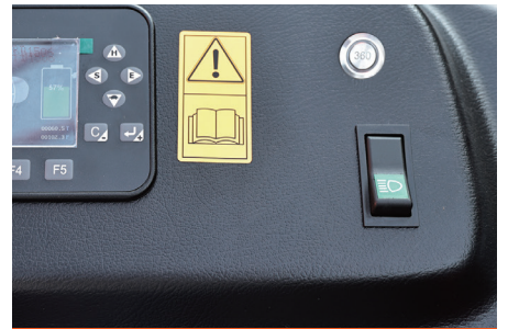
Real-time switching between 180° and 360° steering modes
