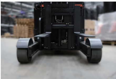
Integrated side shifter
