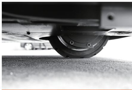
High-clearance 120 mm chassis for better passability
