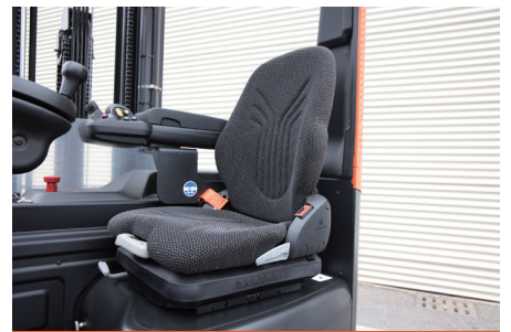
Optional (Grammer) suspension seat with high-elasticity shock absorption
