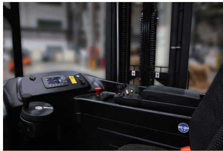
Centralized fingertip control console
