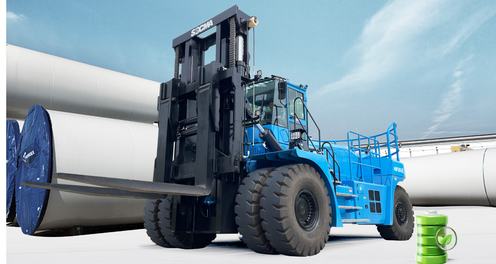
SOCMA HNF-450/500EL electric counterbalance forklift
