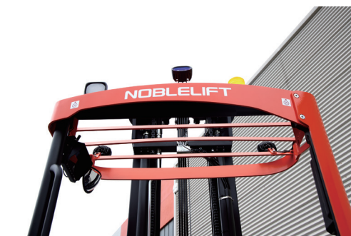
LED lighting and safety blue lights.
