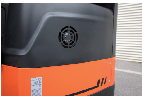
Motor cooling system.
