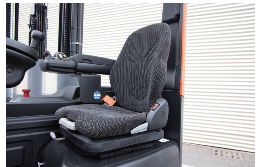
(Grammer) Suspension seat with high-elastic shock absorption.
