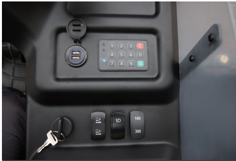
Multi-functional password lock and real-time switching between 180°/360° steering modes.
