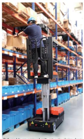
Both models are equipped with automatic closing doors preventing the operation of the truck when doors are opened. High-strength aluminum alloy profiles help to achieve great
