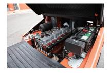
The front and rear floors can be removed by removing two screws on the rear floor.
