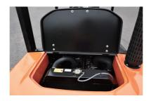
The counterweight top cover opens at a wide angle for easy radiator inspection.
