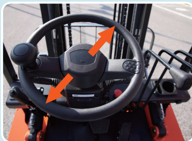
The use of a smaller diameter steering wheel reduces the fatigue for the operator.
