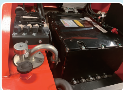
Hydraulic oil level check is convenient.
