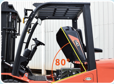
The engine hood opens at an 80-degree angle.
