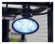
**Blue LED warning lights** The blue LED warning lights enable a visual warning.
